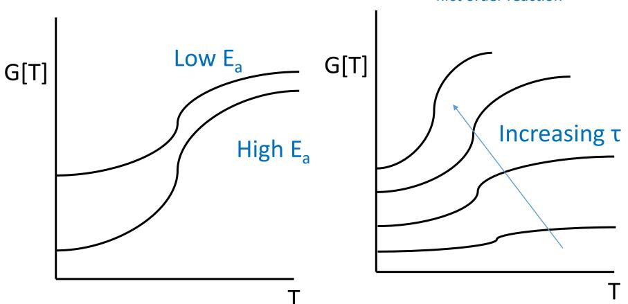
Steady state CSTR solutions are at the intersection of removal and generation terms (when generation exactly equals removal, then there will be no temperature change in time)
