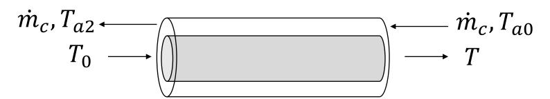
Guess value of  $T_{a2}$ , solve for  $T_{a0}$ . Start with  $T_{a2} = 340 \text{ K}$
