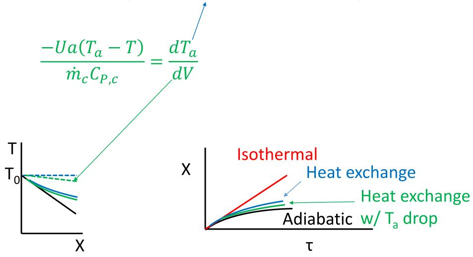
If  $\dot{m}_c C_{P,c}$  is moderate: Once (T<sub>a</sub>-T) is large enough heat removal = gen.! 300 T[V] isothermal 250 — T[V] adiabatic 200 Temperature — T[V] Ua low 150 — T[V] Ua high 100 T[V] co-current Ua low 50 ---- Ta[V] co-current 0 0.3 X[V] isothermal Conversion X[V] adiabatic 0.2 — X[V] Ua low 0.1 — X[V] Ua high X[V] co-current **Ua low** 0.0 0.2 0.4 0.6 8.0 0.0 Volume
