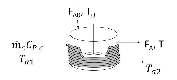
For CSTR, reactor itself is well mixed and uniform temperature, but feed and outlet/reactor may be at different temperatures.
