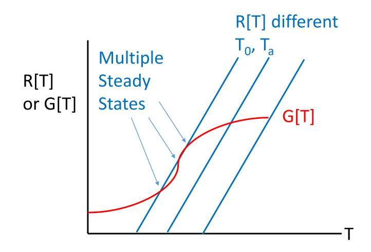
Stability of steady states are based on what occurs with slight perturbations to the reactor temperature.
